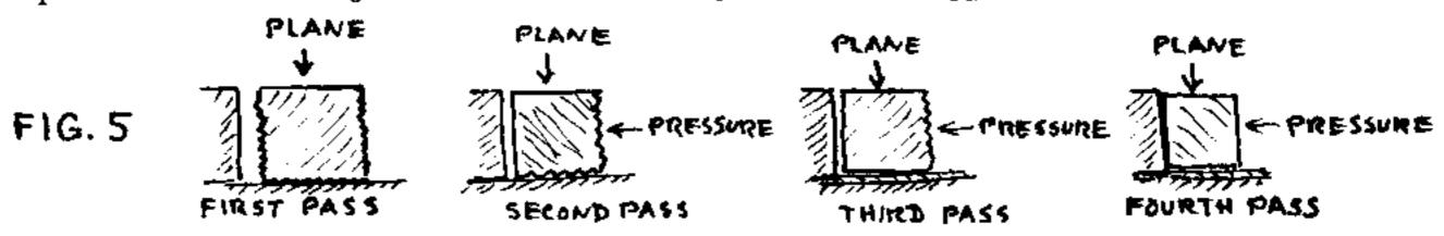
One of the common complaints when planing hardwoods is gouging and splintering of the surface, especially with really difficult woods like bubinga. This has to do with the type of wood, direction of grain, feed speed, speed and sharpness of the cutter, among other factors which you don't have much control over. One thing you can control is the angle at which the knives are ground. The planer blades in most cabinet shops are ground at a so-called "softwood"
